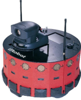
Figure 6: THE MAGELLAN PRO MOBILE ROBOT, WHOSE VISION SYSTEM WAS USED IN THE EXPERIMENTS
