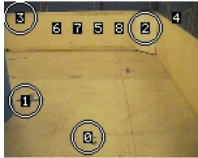
Figure 4.9: Output for the image at the robot’s start position (first exploration loop). The numbers indicate the location of salient points in order of importance (0 corresponds to the most salient) and the white circles indicate that the region corresponding to a particular salient point was considered novel. Because this was the very first image to be presented to the robot, there are several regions that were marked as novel. As the robot explored the arena and the GWR network habituated on it, fewer and fewer regions were labelled as novel.
