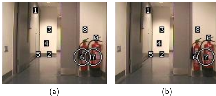
Figure 5.16: False novelty responses for the fire extinguishers: (a) GWR network; (b) incremental PCA. The white circles indicate regions erroneously labelled as novel.
