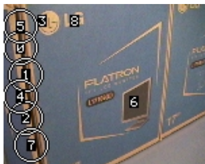
Figure 5.5: Image frame 46 (fifth loop of inspection of the arena with the grey box). A large edge between two cardboard boxes exposes weaknesses regarding feature scale and patch misalignment.
