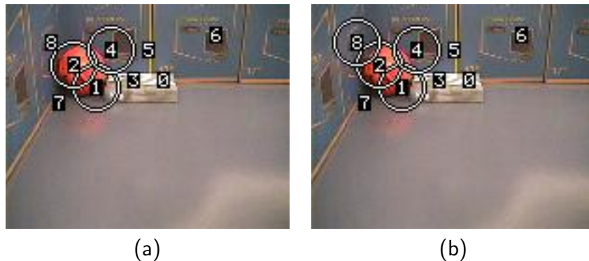
Figure 5.12: Output images for Experiment 13: (a) GWR network; (b) incremental PCA. The orange ball (novel stimulus) is correctly highlighted as novel regardless of the presence of the grey box (normal stimulus).
