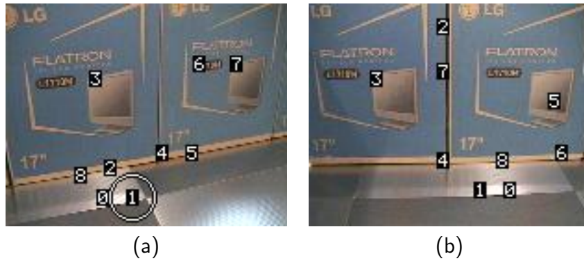
Figure 5.25: Output images for the bright reflection on the floor: (a) during inspection; (b) during exploration. The resulting image patches in the vicinity of regions 1 in (a) and 0 in (b) are noticeably different.
