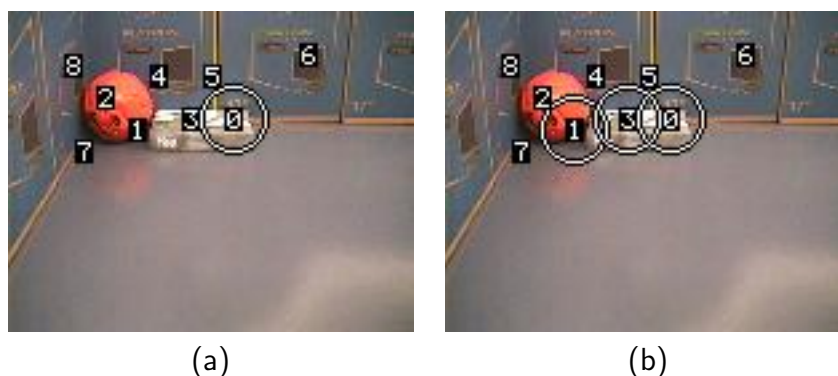
Figure 5.10: Output images for Experiment 12: (a) GWR network; (b) incremental PCA. The grey box (novel stimulus) is correctly highlighted as novel regardless of the presence of the orange ball (normal stimulus).
