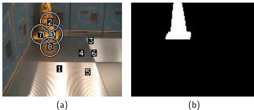
Figure 5.23: Output and ground truth images for the “oval” trajectory inspection when the yellow cone was introduced in the arena. The cone (regions 0, 2 and 7) was correctly identified as being the novel stimulus. Also, the cone’s reflection on the shiny metallic floor (region 8) was highlighted as novel.
