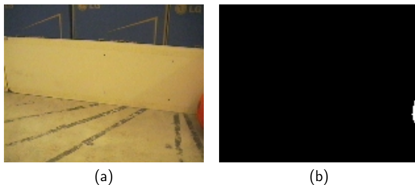
Figure 4.18: Image frame 18 (first loop) and its ground truth novelty map. The area occupied by the orange football corresponds to only 0.55% of the image frame.
