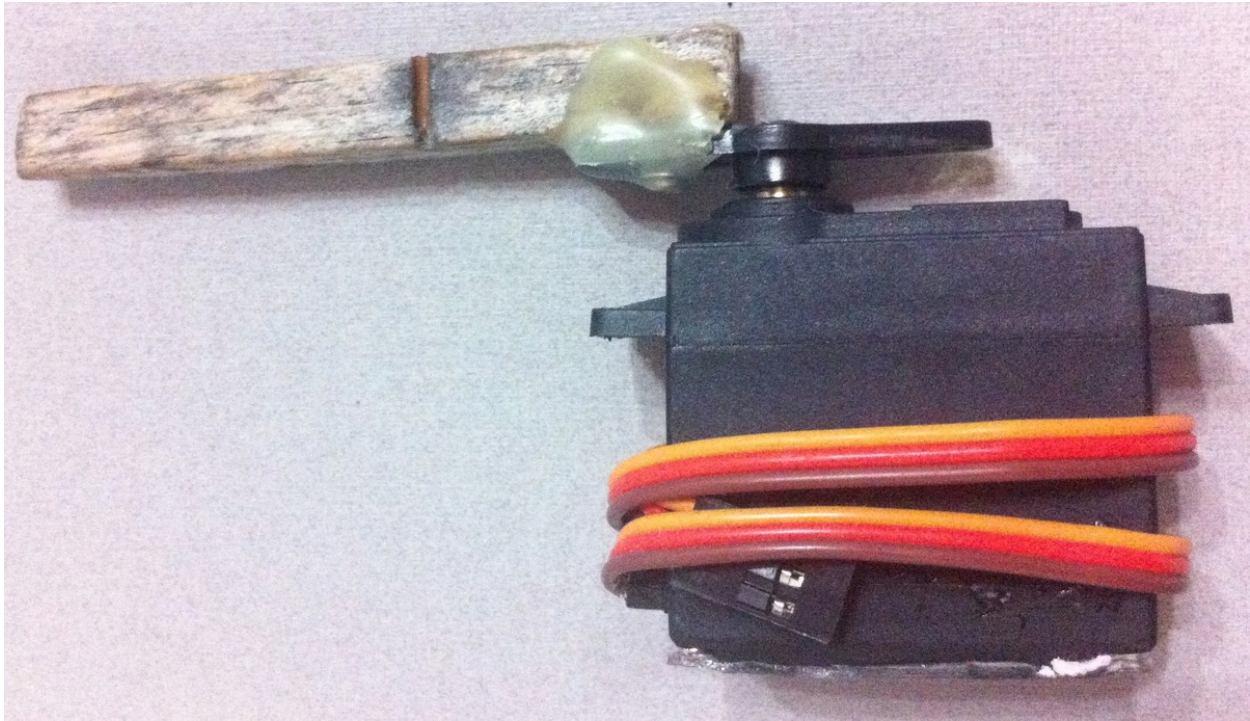
Fig. 3: Hobby servomotor with horns attached to axis used to compress the phantom chambers.
